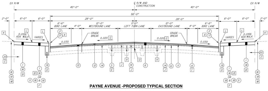
STA 0+10.00 TO STA. 37+30.25 STA 39+53.25 TO STA. 46+42.00 NOTE: 37+30.25 TO STA. 39+53.25 (I-90 UNDERPASS BRIDGE)
